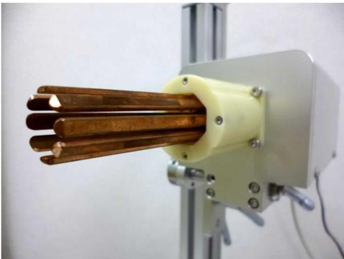
Fig. 1. Instrumentation of the multidirectional lip closing force measurement system
