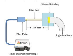
Figure 1. Schema of Fiber Post Transmission Test
